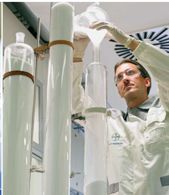
Purification of active substances: Bodo Röhr fills a chromatographic column used for separating substance mixtures and purifying reaction products.
