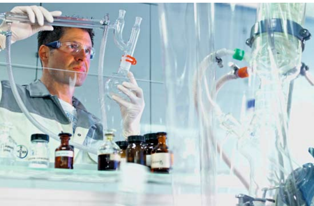
Preparatory work: Frank Kuczynski sets up distillation equipment at the Bayer Schering Pharma research laboratory in Berlin – one of many steps in the synthesis of the new active ingredient sagopilone for test purposes.
