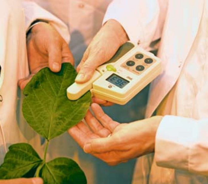
Well distributed: Dr. Isolde Häuser-Hahn checks on an X-ray film whether an experiment with a radioactively labeled compound has succeeded. The colors indicate how the active substance has penetrated into the leaves (left). The chlorophyll content of the plants is also measured (above).
