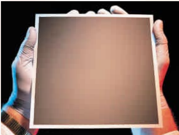
Anode of a 20 x 20 cm SOFC cell.
