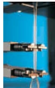
Joachim Peckhaus checks the tensile strength of a plastic part prior to testing.
