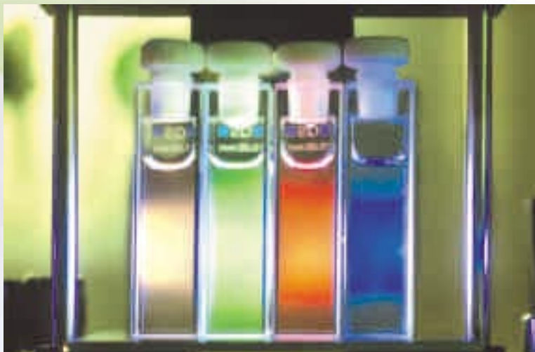
Subjecting the nanophosphors (shown here is a dispersion) to special UV light causes them to fluoresce in different colors.
