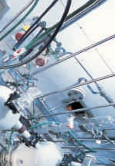
Horst Dieter Botzet inspects the precipitation process used to make plastics electrically conductive.
