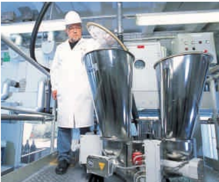
Ralf Hönow fills an extruder for blending the two plastic components.
