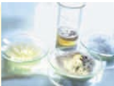
Ingredients: layered silicates and caprolactam are added to the polymerization process to produce the plastic.
