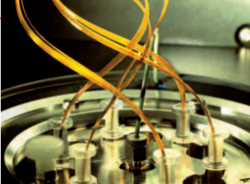
Fiberglass capillaries are used for fragment analysis and also, for example, for separation during DNA sequencing.
