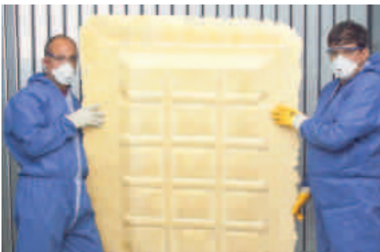
Molded part production: an engine cover for a bus is removed from the mold.
