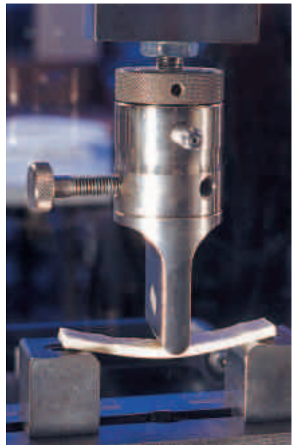
A plastic sample is subjected to a bending test.
