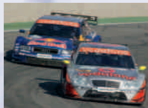
Speedy hot rods: Many of the add-on parts on motor racing vehicles, such as spoilers and side skirts, can be made of glass fiber-reinforced polyurethane.
