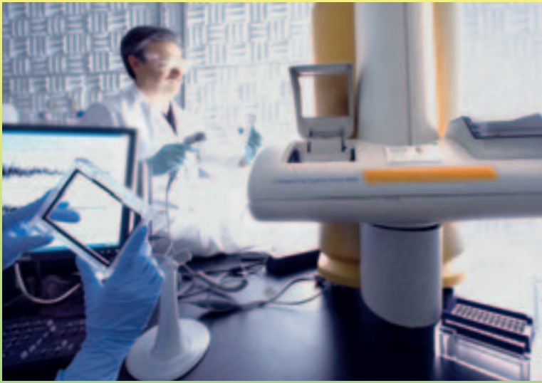
Protein masses: Gary Davis' team examines the composition of thousands of po- tential biomarker proteins in the mass spectrom- eter.
