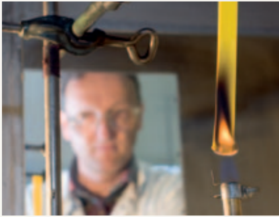
Slow burner: Helmut Wolff tests the new plastic in an open flame.
