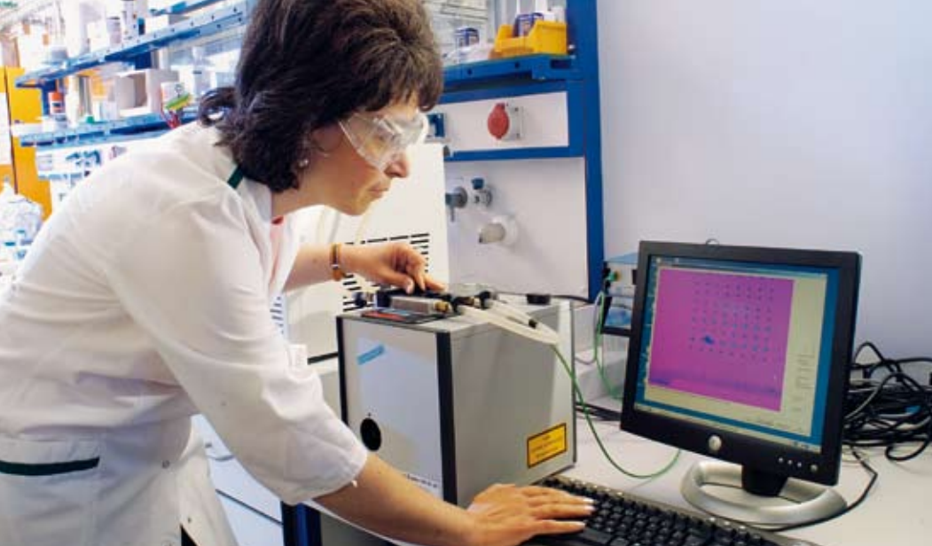
Image analysis: Viktoria Bazilyanska uses the prototype reader to evaluate the mycotoxin assay taken with the biochip. Each of the blue dots on the screen indicates the light intensity of a measurement on the chip.
