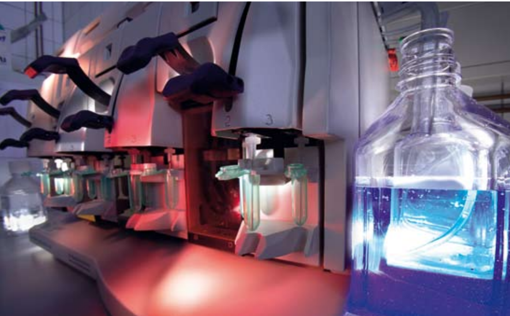
Gene chip test: Ina Flocke prepares the gene chip scanner which can analyze up to 48 chip experiments overnight (right). Beforehand, the chips are cleaned in a washer system to remove dye reagents (left).
