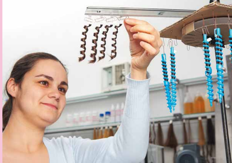
Curl test: Dr. Sophie Viala checks the results of a curl retention test. The test shows how well hair sprayed with hair spray containing the new PU molecule retains its curl in moist air.
