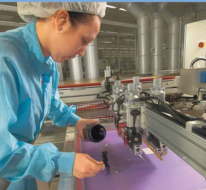
Flexible mini power plants: organic photovoltaics contain several layers of ultrathin materials that are only tens of nanometers thick. Melanie Treichel prepares the printing procedure for this in clean-room conditions (photo left). The flexible film sandwich (photo right) can be easily formed into different shapes.
