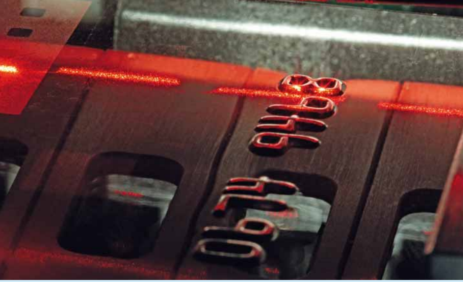
Test station: the ProteXXion® security system uses a laser (photo above) to scan the metal platelets embedded in the film before comparing this pattern with the one in the database. Lab technician Kira Planken (photo right) reviews the quality of the transparent Makrofol® plastic film used in this application; it is only about 100 micrometers thick.
