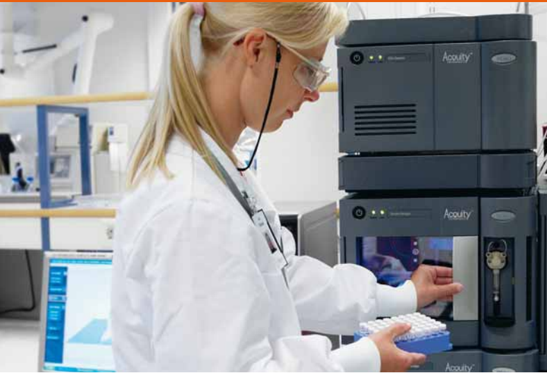
Materials development: Bayer HealthCare employee Satu Raitala prepares the liquid chromatograph for a chemical analysis of the new intrauterine system.
