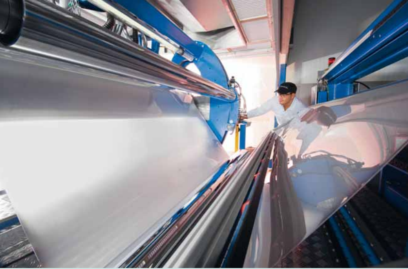
High-tech light on a roll: Erkan Bozkurt monitors the manufacture of the wafer-thin Makrofol® films for the OLEDs on an extrusion machine (photo, left). The effects that elevated temperatures and humidity have on the ageing process of the illuminating films are investigated by Alexander Pogorzalek in a special test chamber at Bayer MaterialScience in Leverkusen (photo, right).
