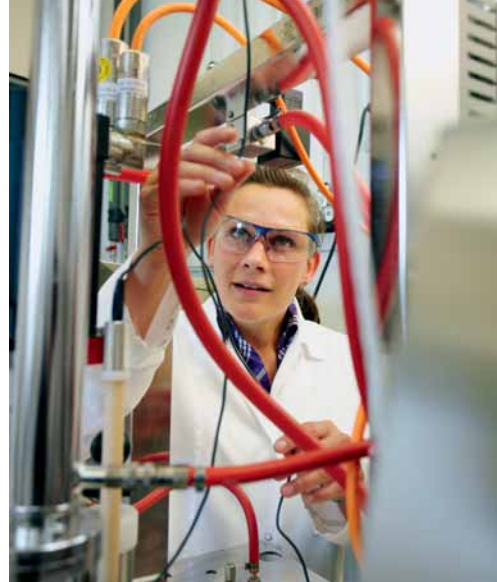
A sharp-eyed biochemist: laboratory manager Dr. Ulrike Hänsel checks the tubes supplying the bacteria in the fermenter with the ideal amounts of oxygen and the other nutrients they need.
