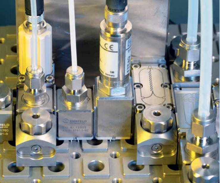
The heart of the new process: one approach for transferring production to a continuous procedure involves the use of microreactors, where the substance can react much faster and more efficiently (photo, left). Dr. Agathe Christine Mayer and Dr. Gerhard Braun (photo, right, left to right) first developed the production method in their automated parallel reactors in the laboratory. The process is now being transferred to a demonstration plant for active ingredient production.
