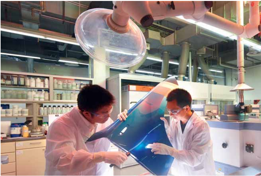
Quality control – if the aim is to make cars lighter by using plastics, innovative approaches to coating are required. Laboratory engineers Michael Chen (left) and Daogui Li (right) assess a freshly coated fender at Bayer MaterialScience's Shanghai research center.
