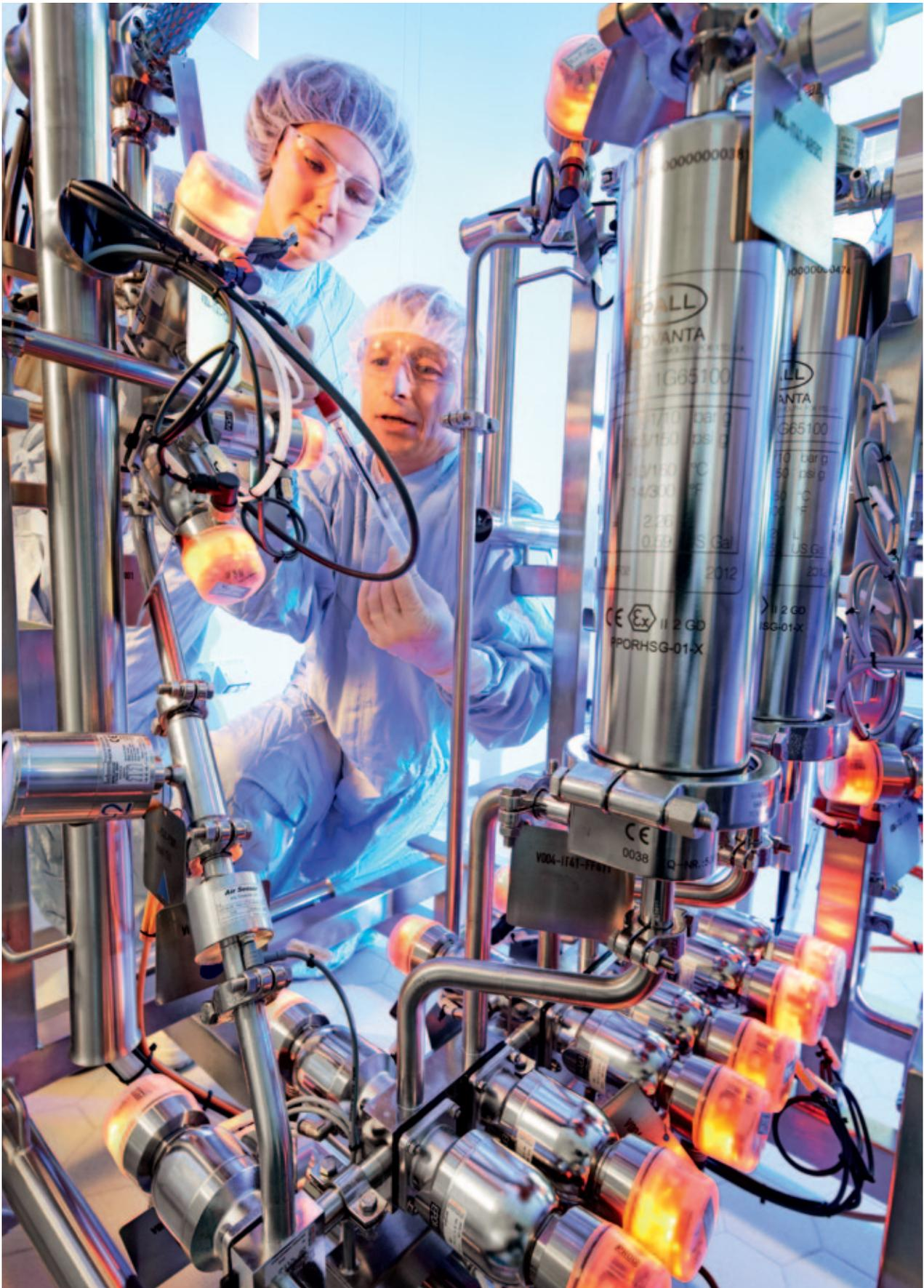
Optimum process chain: Jennifer Tummes (left) and Philipp Ehrsam check a pH sensor on the fermenter in which cells produce biologics.
