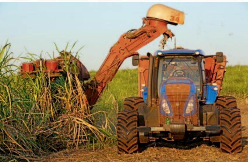
Harvest under control: Brazil's state-of-the-art sugarcane harvesting machines are GPS-controlled to prevent unnecessary destruction of soil or yields
