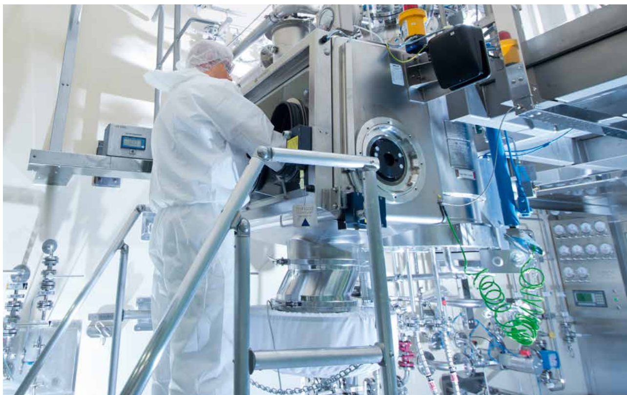
The purity law: Adam Mikolasch uses a continuous tube system that transports the highly potent active ingredient through a dust-free and hermetically sealed environment to final packaging.
