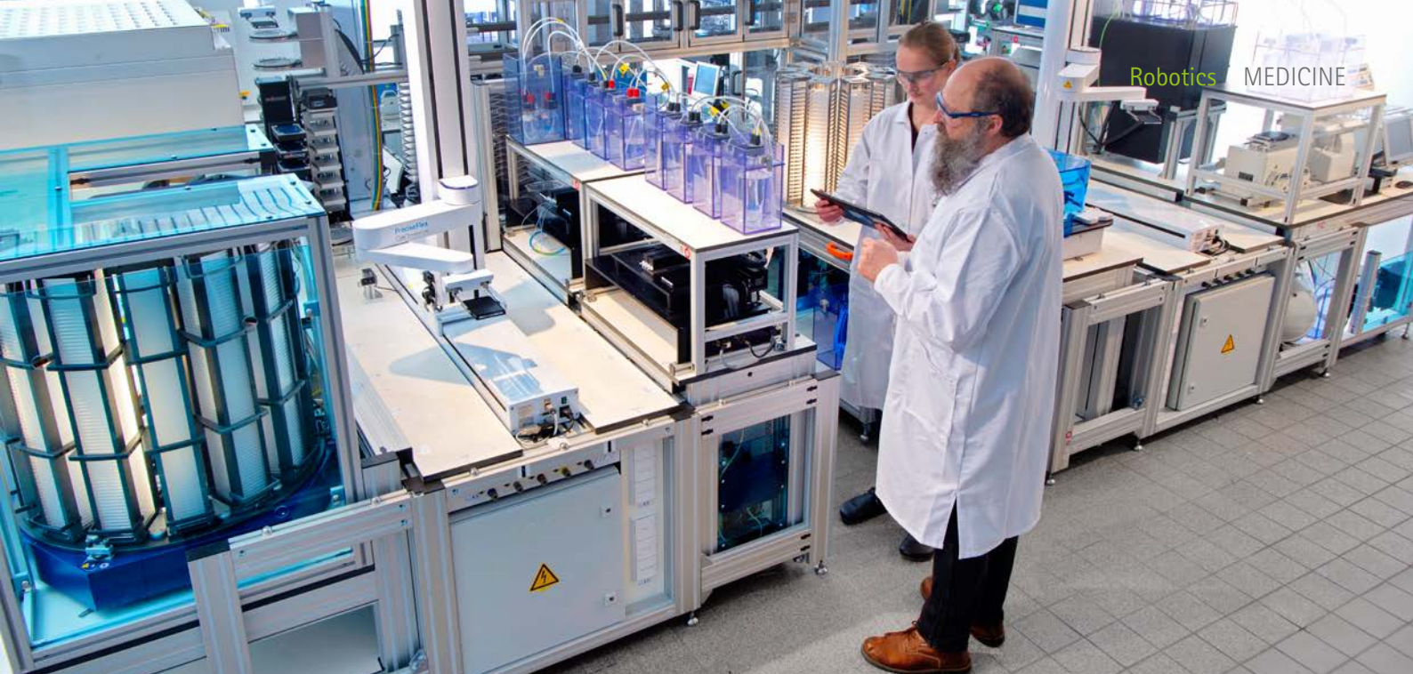
A four-armed octopus: the unique system can screen Bayer's entire substance library, containing 4.1 million molecules, within a few days. The octopus was constructed by Bayer employee Georg Schmidt, shown standing with colleague Maïke Günther.
