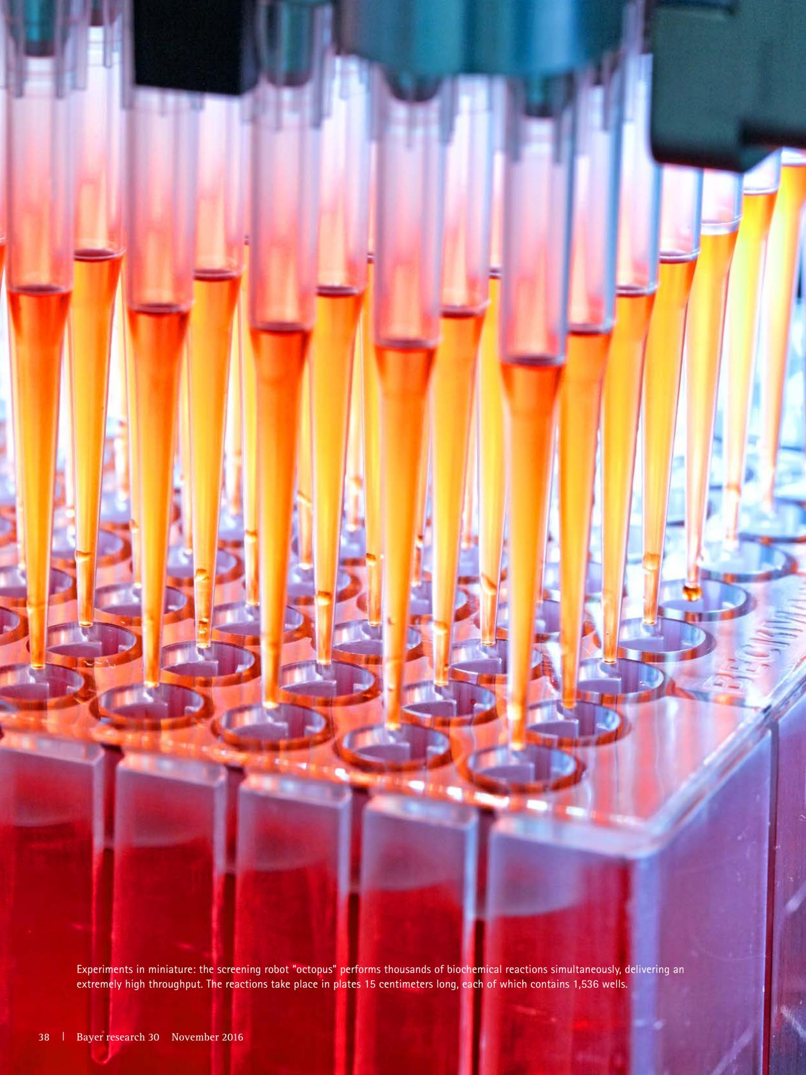
Experiments in miniature: the screening robot "octopus" performs thousands of biochemical reactions simultaneously, delivering an extremely high throughput. The reactions take place in plates 15 centimeters long, each of which contains 1,536 wells.
